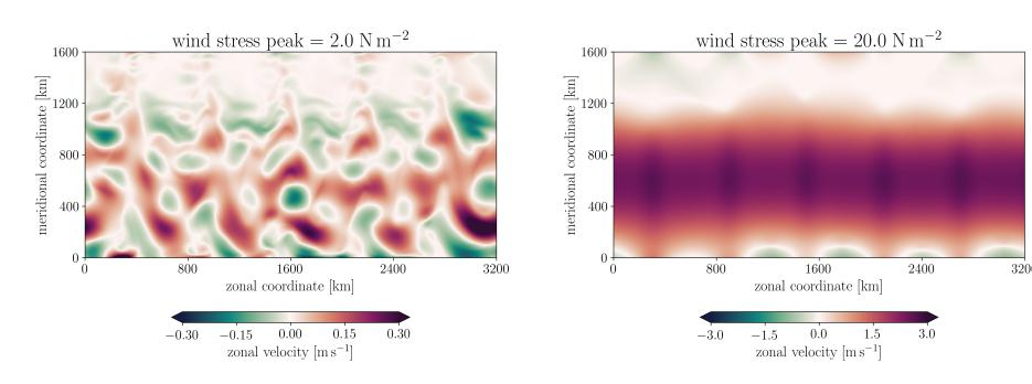
[zonal flow structure for 1-layer setup]
