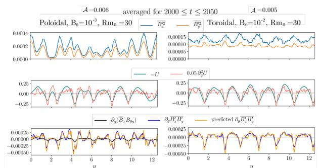
Maxwell stress are well approximated as "magnetic viscosity" through eq. (1) [with  $\alpha \approx 1$ ].
