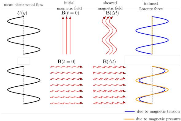
[Magnetic response to a mean shear flow expected in turbulent regime]
