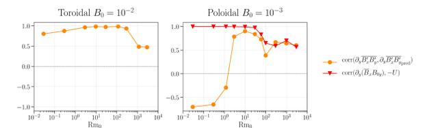
As we cross  $Rm_0 = 1$  the Lorentz force transitions from magnetic drag ( $\propto -U$ ) to magnetic viscosity ( $\propto \partial_y^2 U$ ).
