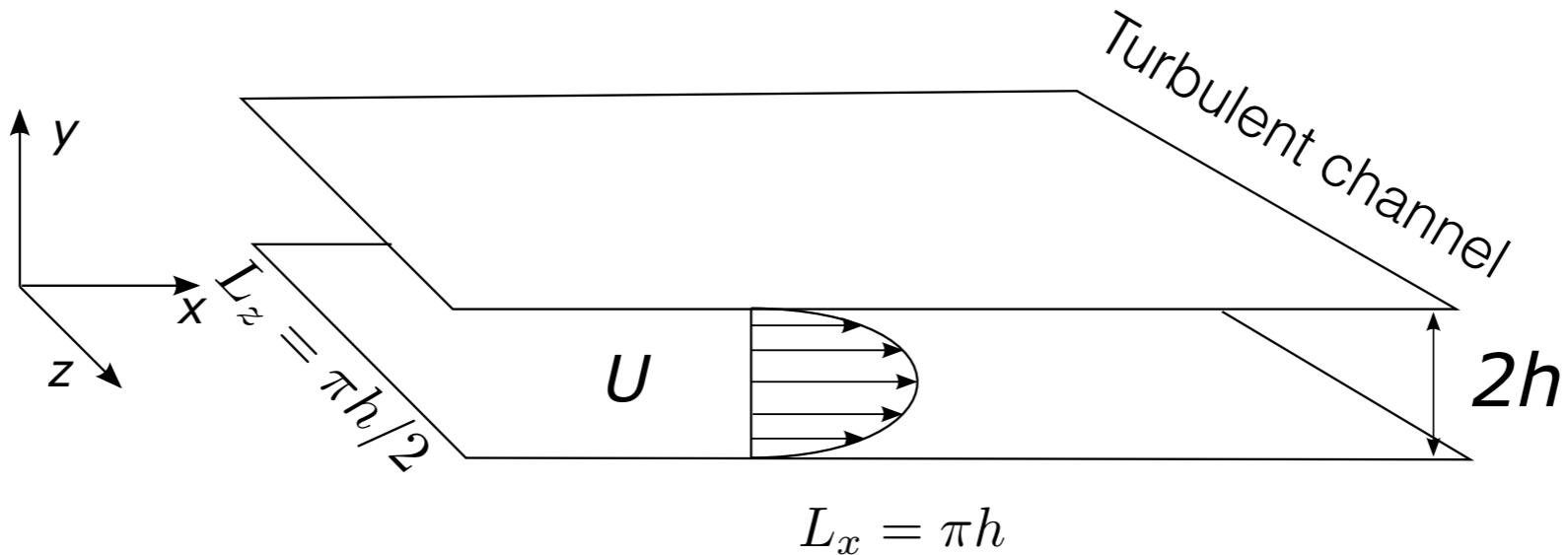
$$\begin{aligned} \mathbf{u}(x, y, z, t) &= \bar{\mathbf{u}}(y, z, t) + \mathbf{u}'(x, y, z, t) \\ &\text{streamwise mean} \quad + \quad \text{perturbations} \end{aligned}$$
