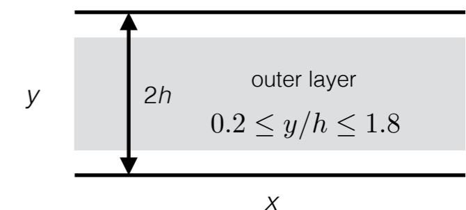
$$\frac{dQ}{dt} = \left( \begin{array}{l} \text{cross-stream advection} \\ \text{of } \bar{\omega}_x^2 \text{ into outer layer} \\ \text{due to roll } (\bar{v}, \bar{w}) \end{array} \right) + \left( \begin{array}{l} \text{Reynolds stress torque} \\ \text{production in outer layer} \\ \text{due to } \mathbf{u}' \end{array} \right) + \left( \text{dissipation} \right)$$
