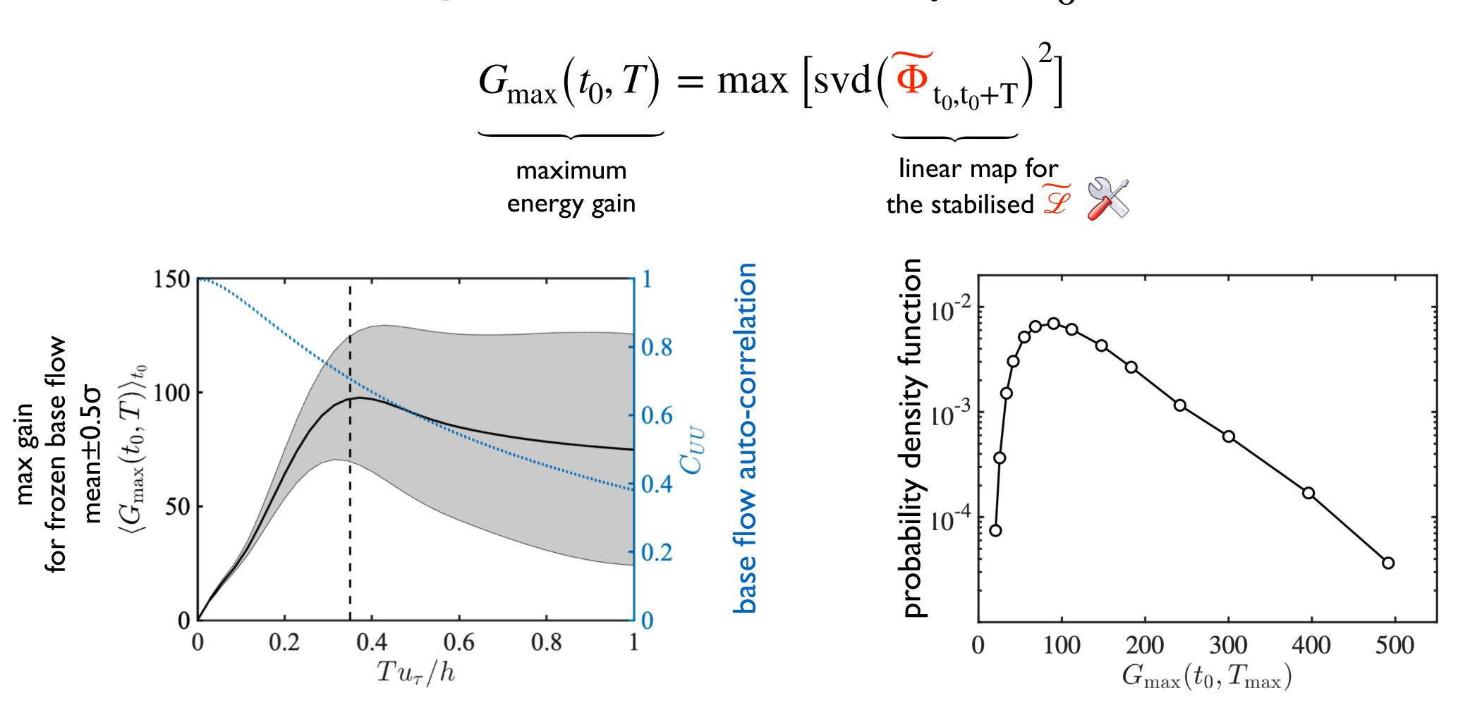
[Note that streaky base flow  $U(y, z, t_0)$  gives gains O(100). Base flows U(y) induce gain O(10).]
