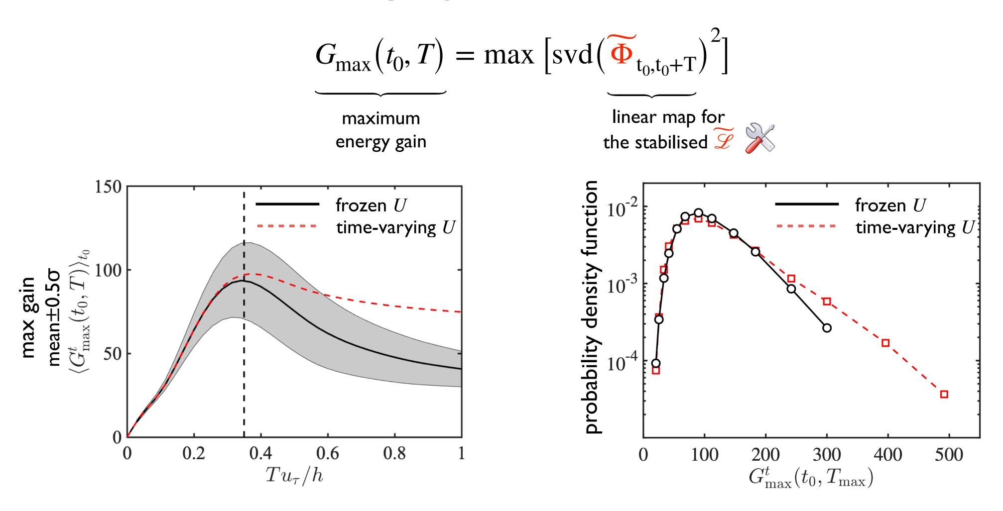
Time-variability of the base flow U(y,z,t) does not enhance energy transfer to fluctuations for short times.
