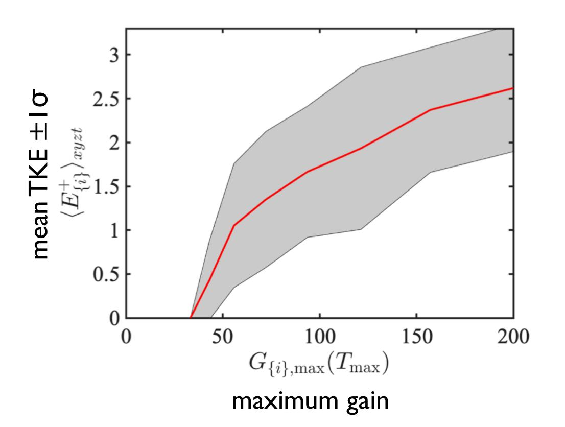
frozen base flows  $U(y, z, t_i)$ with gain  $\gtrsim 40$ sustain turbulence
