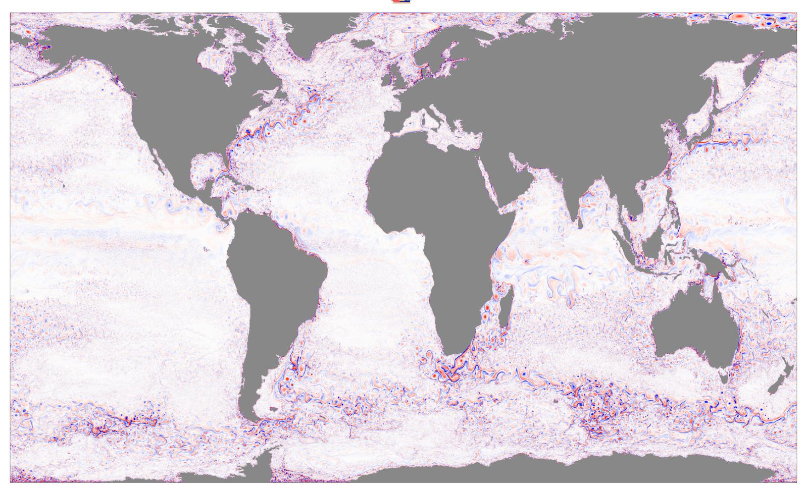
near-global (75°S-75°N) ocean simulation at 1/12° horizontal resolution, 48 vertical levels @ 68 Nvidia A100 achieving 10 simulated years per day
